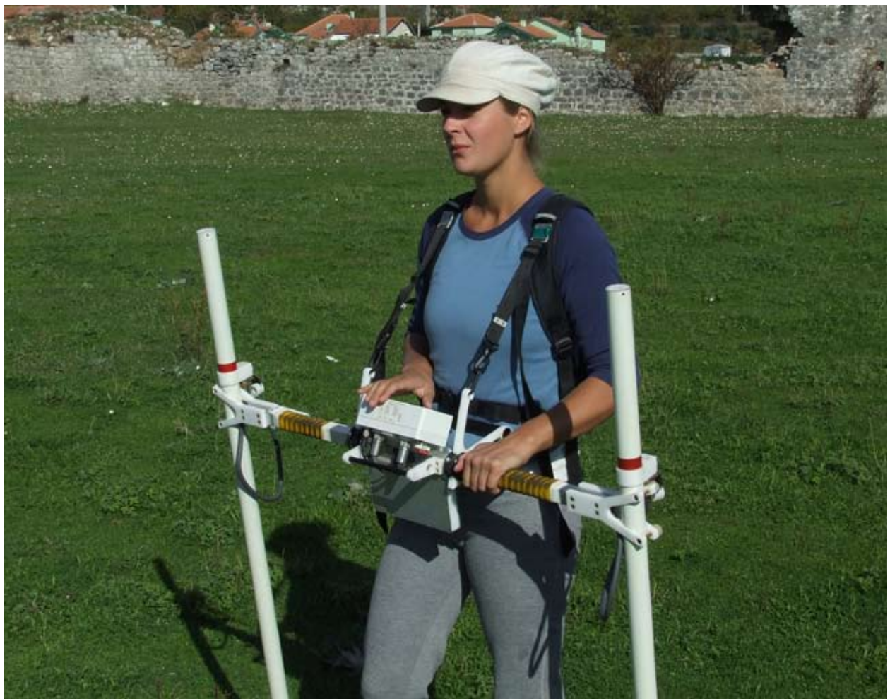
Plate. 3 : Bartington Grad 601-2 with operator (photo: S.Hay)
