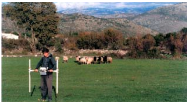
Plate. 8: Setting the parameters and balancing the Bartington Grad 601-2 at Doclea (photo: S.Hay)
